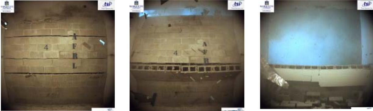
*Unprotected walls can collapse and send dangerous debris into building.*
